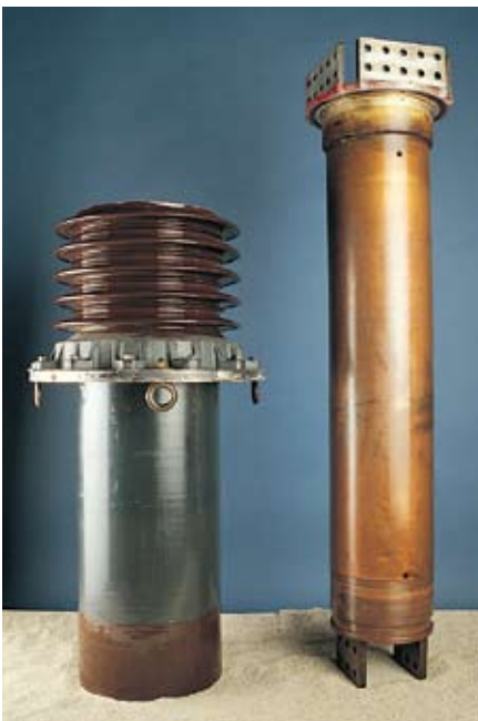
Conductive Ink Moves From Conductive Layer (A) To Insulating Layer (B) Within Bushing Core.
